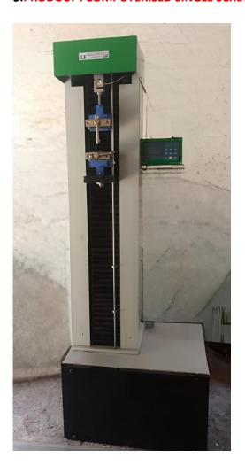
UNIVERSAL TENSILE MACHINE: (TENSILE/ELONGATION/FLEXURAL/COMPRESSION/PEAK LOAD/AVERAGE LOAD/PEEL/BOND TESTER) AS PER STANDARD
